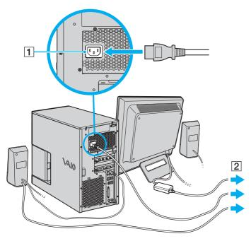
To disconnect the computer completely from AC power, unplug the power cord.
